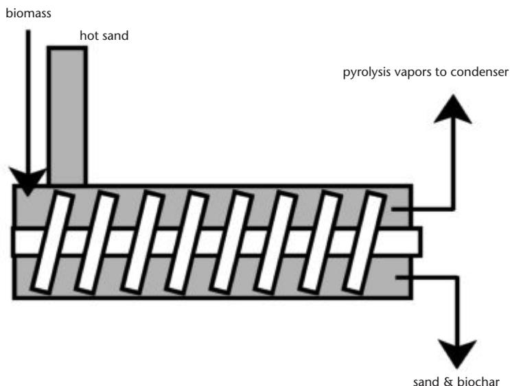
**Figure 1c.** An auger reactor uses a heated tube where biomass and sand enter and move through the tube via the auger rotation. The biomass is continually fed into the cylinder with no oxygen, and is heated to temperatures high enough for pyrolysis to occur. Volatiles are collected and condensed to oils. Char and sand are collected at the end of the auger. Auger reactors are relatively simple designs and can be scaled up to larger reactor sizes.
